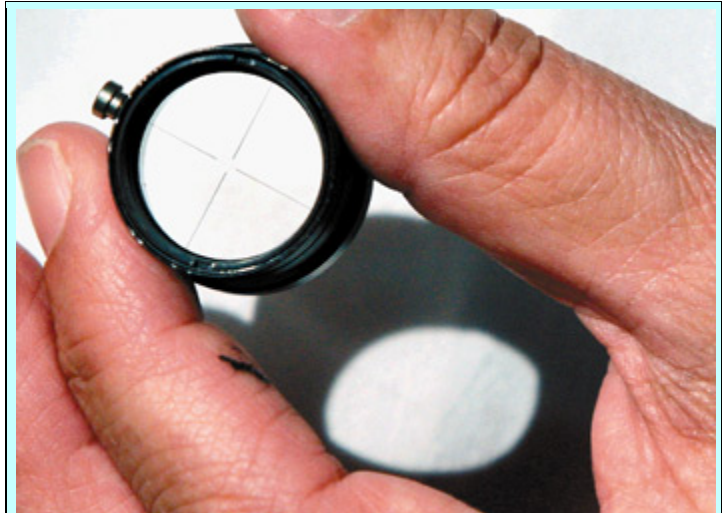
High-quality reticles for a rifle scope are checked for dirt and flaws at Premier Reticles. Reticles are crosshairs, fine lines, and dots that create a focal point on an eyepiece. The 63-year-old company is now moving beyond reticles to designing and producing rifle scopes. Photo by Jeff Taylor
